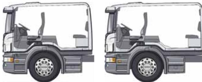
The Scania CrewCab is available in a long and a short version for 4-5 and 6-8 passengers respectively. The cabs are all-steel and based on regular Scania cab components.
