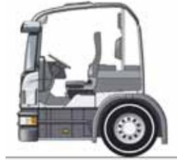
Scania's low-entry cab is mounted low on the chassis. The bottom boarding step is 155 mm off the ground when the truck is kneeling. The cab has convenient cross-cab access and seating capacity for up to 4 persons. The all-steel cab is based on regular Scania cab components.
