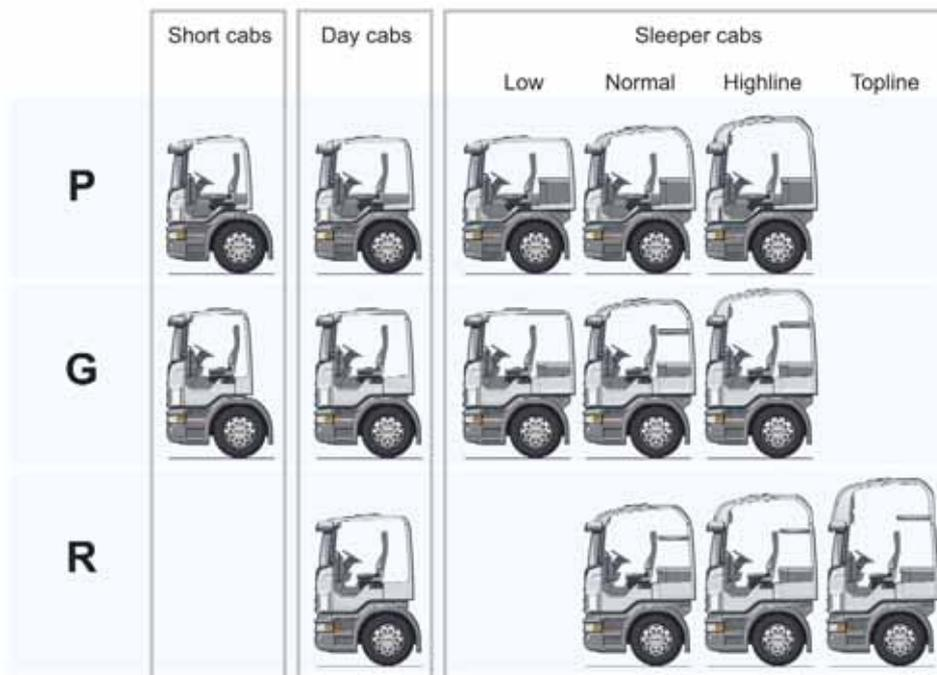
The introduction of a Highline version extends the suitability of the P-series to regional long-haulage. All Highline models get a new roof shelf with closed storage above the windscreen.
