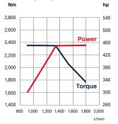
**9-litre, 360 hp** Biodiesel, HVO, diesel
