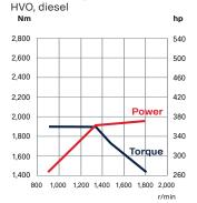
**9-litre, 360 hp** Biodiesel, HVO, diesel
