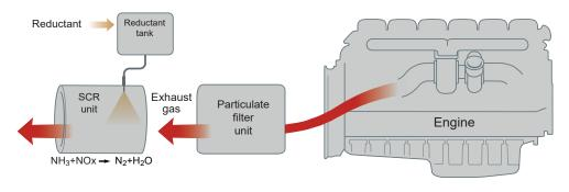
The emissions of particulate matter are filtered through a ceramic structure, that only allows particles smaller than a defined size to pass. When the filter is filled with soot particles to a specific amount, it is regenerated automatically.
