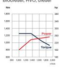
9-litre, 310 hp Biodiesel, HVO, diesel
