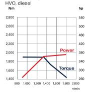
9-litre, 360 hp Biodiesel, HVO, diesel
