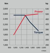
**9-litre, 360 hp** Biodiesel, HVO, diesel
