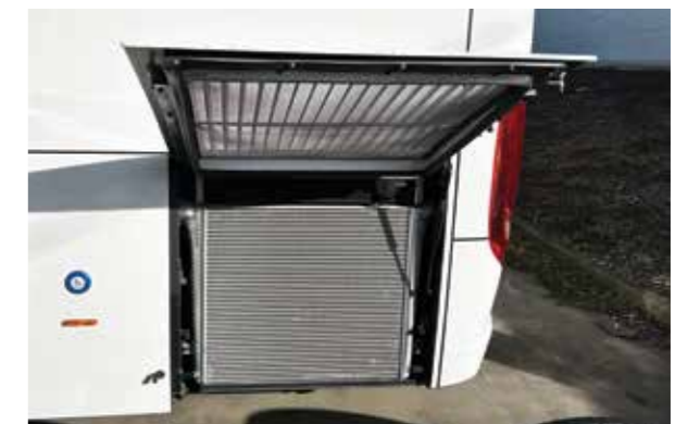
Swing open intercooler door for easy access and maintenance.
