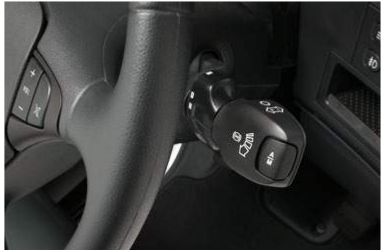
Location of Retarder and Opticruise control by the steering wheel.
