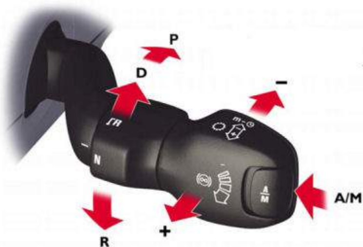
Function description of Opticruise and Retarder, controlling by the steering wheel
