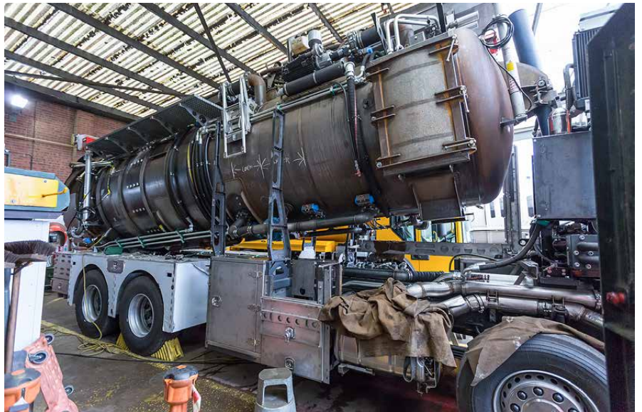
Inside the huge vacuum tanker, which needed a specially-adapted Scania chassis to carry it.
