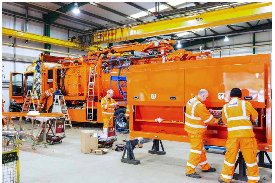
Hydro's crew equips 'Terminator'. The tanker sits over drains and extend long, flexible pipes up to 80 metres down into sewers, drawing up liquid waste by creating a vacuum in the tank. It cleans the water before recycling much of it back into the system.
