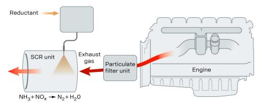
The emissions of particulate matter are filtered through a ceramic structure, that only allows particles smaller than a defined size to pass. When the filter is filled with soot particles to a specific amount, it is regenerated automatically.
