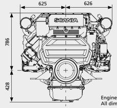
Engine with heat exchanger All dimensions in mm
