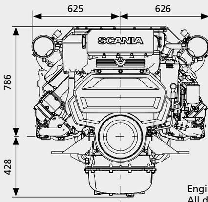
Engine with heat exchanger
