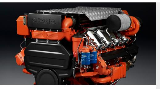
The marine engines from Scania are based on a robust design with a strength optimized cylinder block containing wet cylinder liners that can easily be exchanged. Individual cylinder heads with 4 valves per cylinder promotes repairability and fuel economy. The engines are type-approved in all major classification societies.
