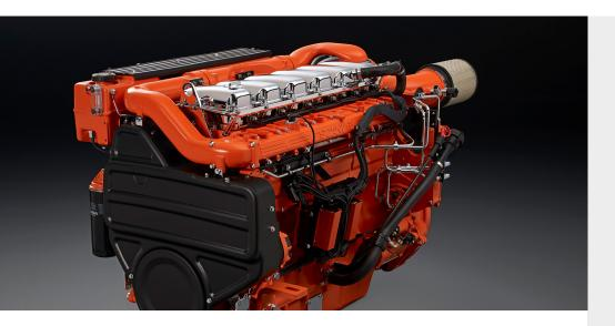
The marine engines from Scania are based on a robust design with a strength optimized cylinder block containing wet cylinder liners that can easily be exchanged. Individual cylinder heads with 4 valves per cylinder promotes reparability and fuel economy. The engines are type-approved in all major classification societies.
