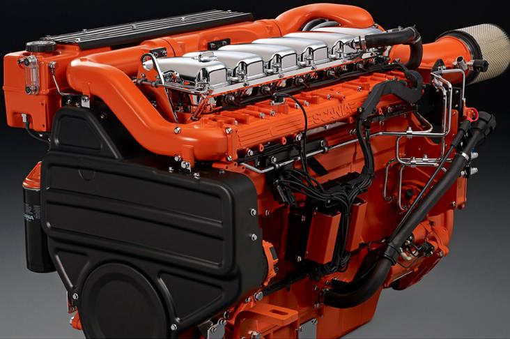
The marine engines from Scania are based on a robust design with a strength optimized cylinder block containing wet cylinder liners that can easily be exchanged. Individual cylinder heads with 4 valves per cylinder promotes reparability and fuel economy. The engines are type-approved in all major classification societies.
