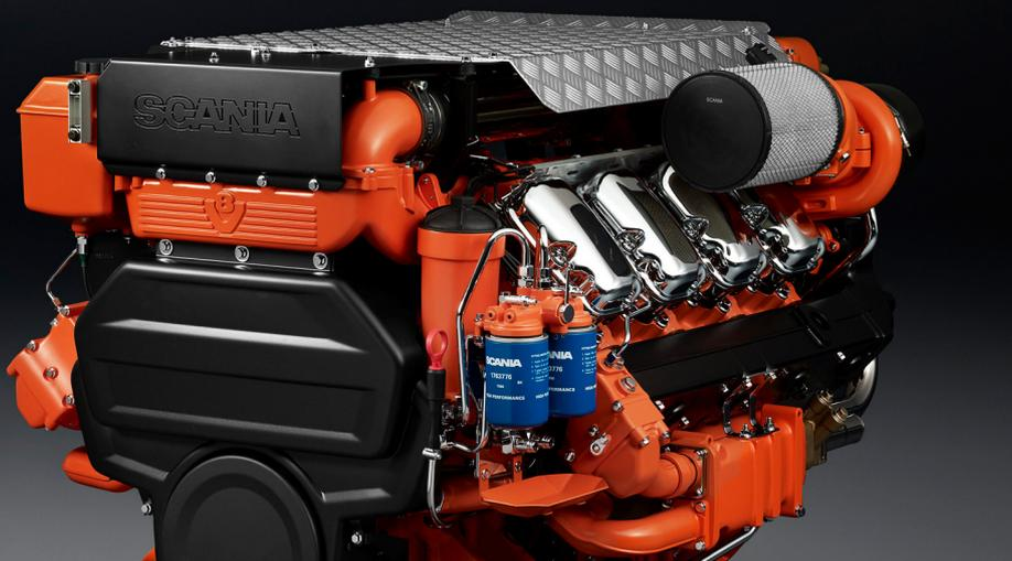
The marine engines from Scania are based on a robust design with a strength optimised cylinder block containing wet cylinder liners that can easily be exchanged. Individual cylinder heads with 4 valves per cylinder promotes reparability and fuel economy. The engines are type approved in all major classification societies.
