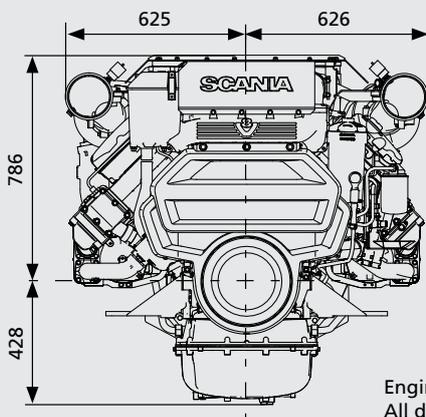
Engine with heat exchanger
