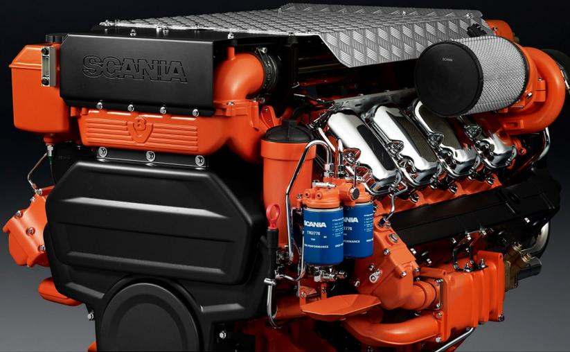
The marine engines from Scania are based on a robust design with a strength optimised cylinder block containing wet cylinder liners that can easily be exchanged. Individual cylinder heads with 4 valves per cylinder promotes reparability and fuel economy. The engines are type approved in all major classification societies.
