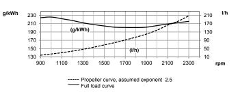
Test conditions Air temperature +25°C. Barometric pressure 100 kPa (750 mmHg). Humidity 30 %. Diesel fuel acc. to ECE R 24 Annex 6. Density of fuel 0.840 kg/dm³. Viscosity of fuel 3.0 cSt at 40°C. Energy value 42700 kJ/kg. Power test code ISO 3046. Power and fuel values +/-3%.
