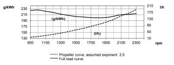
Test conditions Air temperature +25°C. Barometric pressure 100 kPa (750 mmHg). Humidity 30 %. Diesel fuel acc. to ECE R 24 Annex 6. Density of fuel 0.840 kg/dm³. Viscosity of fuel 3.0 cSt at 40°C. Energy value 42700 kl/kg. Power test code ISO 3046. Power and fuel values +/-3%.
