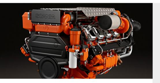
The marine engines from Scania are based on a robust design with a strength optimised cylinder block containing wet cylinder liners that can easily be exchanged. Individual cylinder heads with 4 valves per cylinder promotes reparability and fuel economy. The engines are also available as type-approved with jacketed fuel pipes.
