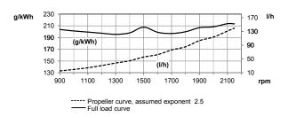
Test conditions Air temperature +25°C. Barometric pressure 100 kPa (750 mmHg). Humidity 30 %. Diesel fuel acc. to ECE R 24 Annex 6. Density of fuel 0.840 kg/dm². Viscosity of fuel 3.0 cSt at 40°C. Energy value 42700 kJ/kg. Power test code ISO 3046. Power and fuel values +/-3%.
