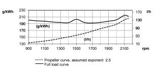
Test conditions Air temperature +25°C. Barometric pressure 100 kPa (750 mmHg). Humidity 30 %. Diesel fuel acc. to ECE R 24 Annex 6. Density of fuel 0.840 kg/dm². Viscosity of fuel 3.0 cSt at 40°C. Energy value 42700 kJ/kg. Power test code ISO 3046. Power and fuel values +/-3%.
