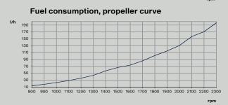
**Test conditions.** Air temperature +25 °C. Barometric pressure 100 kPa (750 mmHg). Humidity 30%. Diesel fuel acc.to ECE R 24 Annex 6. Density of fuel 0,840 kg/dm³. Viscosity of fuel 3.0 cSt at 40 °C. Energy value 42,700 kJ/kg. **Power test code** ISO 3046. Power and fuel values +/-3%.
