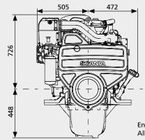
Engine with heat exchanger All dimensions in mm
