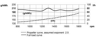
Test conditions Air temperature +25°C. Barometric pressure 100 kPa (750 mmHg). Humidity 30 %. Diesel fuel acc. to ECE R 24 Annex 6. Density of fuel 0.840 kg/dm². Viscosity of fuel 3.0 cSt at 40°C. Energy value 42700 kJ/kg. Power test code ISO 3046. Power and fuel values +/-3%.
