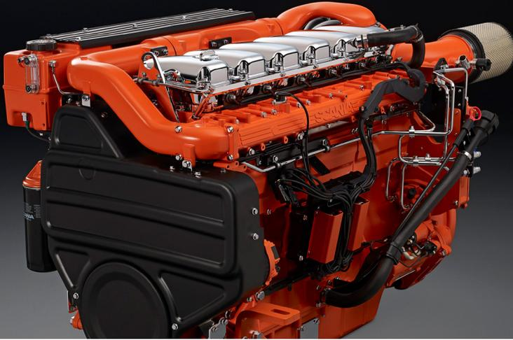
The marine engines from Scania are based on a robust design with a strength optimised cylinder block containing wet cylinder liners that can easily be exchanged. Individual cylinder heads with 4 valves per cylinder promotes reparability and fuel economy. The engines are type approved in all major classification societies.
