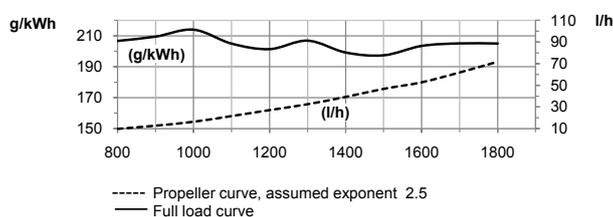
Test conditions Air temperature +25°C. Barometric pressure 100 kPa (750 mmHg). Humidity 30%. Diesel fuel acc. to ECE R 24 Annex 6. Density of fuel 0.840 kg/dm<sup>3</sup>. Viscosity of fuel 3.0 cSt at 40°C. Energy value 42700 kJ/kg. Power test code ISO 3046. Power and fuel values +/-3%.
