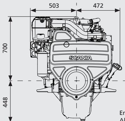
Engine with heat exchanger
