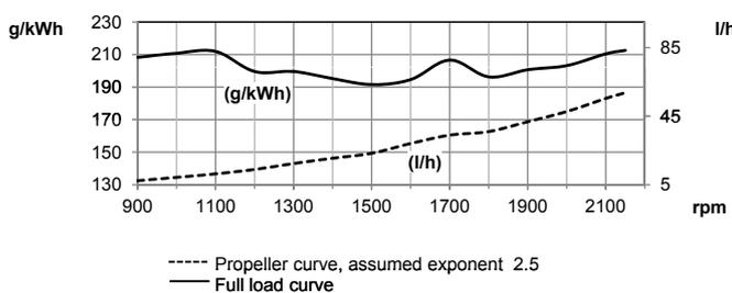
Test conditions Air temperature +25°C. Barometric pressure 100 kPa (750 mmHg). Humidity 30%. Diesel fuel acc. to ECE R 24 Annex 6. Density of fuel 0.840 kg/dm<sup>3</sup>. Viscosity of fuel 3.0 cSt at 40°C. Energy value 42700 kJ/kg. Power test code ISO 3046. Power and fuel values +/-3%.
