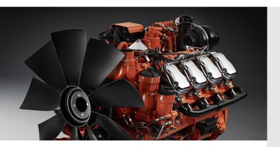
The industrial engines from Scania are based on a robust design with a strength optimised cylinder block containing wet cylinder liners that can easily be exchanged. Individual cylinder heads with 4 valves per cylinder promotes repairability and fuel economy.
