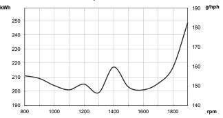
Test conditions Air temperature +25°C. Barometric pressure 100 kPa (750 mmHg). Humidity 30 %. Diesel fuel acc. to ECE R 24 Annex 6. Density of fuel 0.840 kg/dm². Viscosity of fuel 3.0 cSt at 40°C. Energy value 42700 kJ/kg. Power test code ISO 3046. Power and fuel values +/-3%.
