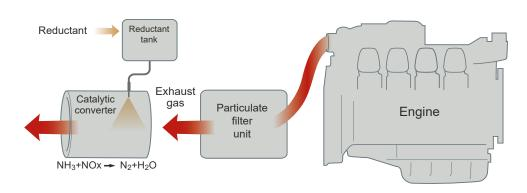
The emissions of particulate matter are filtered through a ceramic structure, that only allows particles smaller than a defined size to pass. When the filter is filled with soot particles to a specific amount, it is regenerated automatically.
