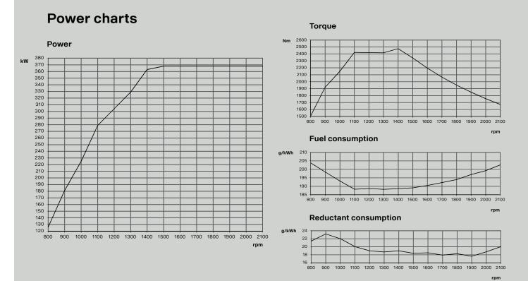
Test conditions. Air temperature +25 °C. Barometric pressure 100 kPa (750 mmHg). Humidity 30%. Diesel fuel acc.to ECE R 24 Annex 6. Density of fuel 0,840 kg/dm<sup>3</sup>. Viscosity of fuel 3.0 cSt at 40 °C. Energy value 42,700 kJ/kg. Power test code ISO 3046. Power and fuel values +/-3%.
