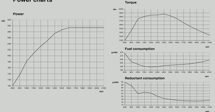
Test conditions. Air temperature 25°C. Barometric pressure 100 kPa (750 mmHg). Humidity 30%. Diesel fuel acc.to ECE R 24 Annex 6. Density of fuel 0.84 kg/dm<sup>3</sup>. Viscosity of fuel 3.0 cSt at 40°C. Energy value 42,700 kJ/kg. Power test code ISO 3046. Power and fuel values ±3%.
