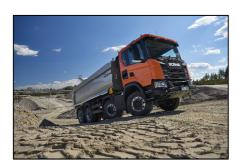
With XT, Scania is introducing a model for the most challenging assignments, where characteristics such as robustness, productivity and uptime are crucial. The powerful bumper protrudes 150 millimetres, and along with a skid plate and headlamp protection mesh provides effective protection for the front of the vehicle in the event of minor impacts.
