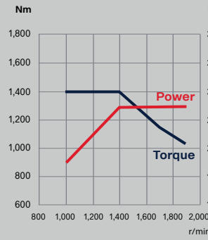
13-litre, 410 hp Biodiesel, HVO, diesel
