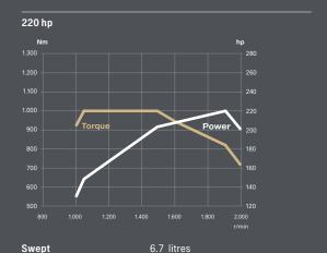
Swept 220 hp (164 kW) at 1,900 r/min Maximum power: 1,000 Nm between 1,050 and 1,500 r/min Maximum torque:
