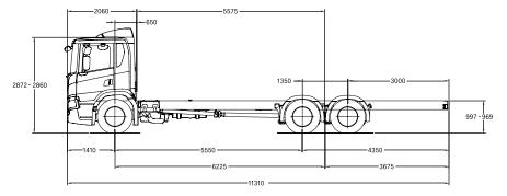
Turntable mounting angles protrude 40 mm above the chassis.
