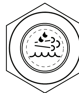
Warning lamp for low reductant level
