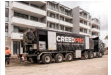
« Eye-catching combination: The Screepro truck and trailer turns heads across Australia. The P 380s were carefully specified to be ideally suited to the job of pulling and powering the imported trailers. The steerable axles on the trailers assist in gaining access to the tightest of locations, as the image below left attests.
