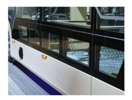
Additional windows For the low floor variant, customers can select an additional lower side windows between the front and rear axle, which adds even more light in the passenger area.
