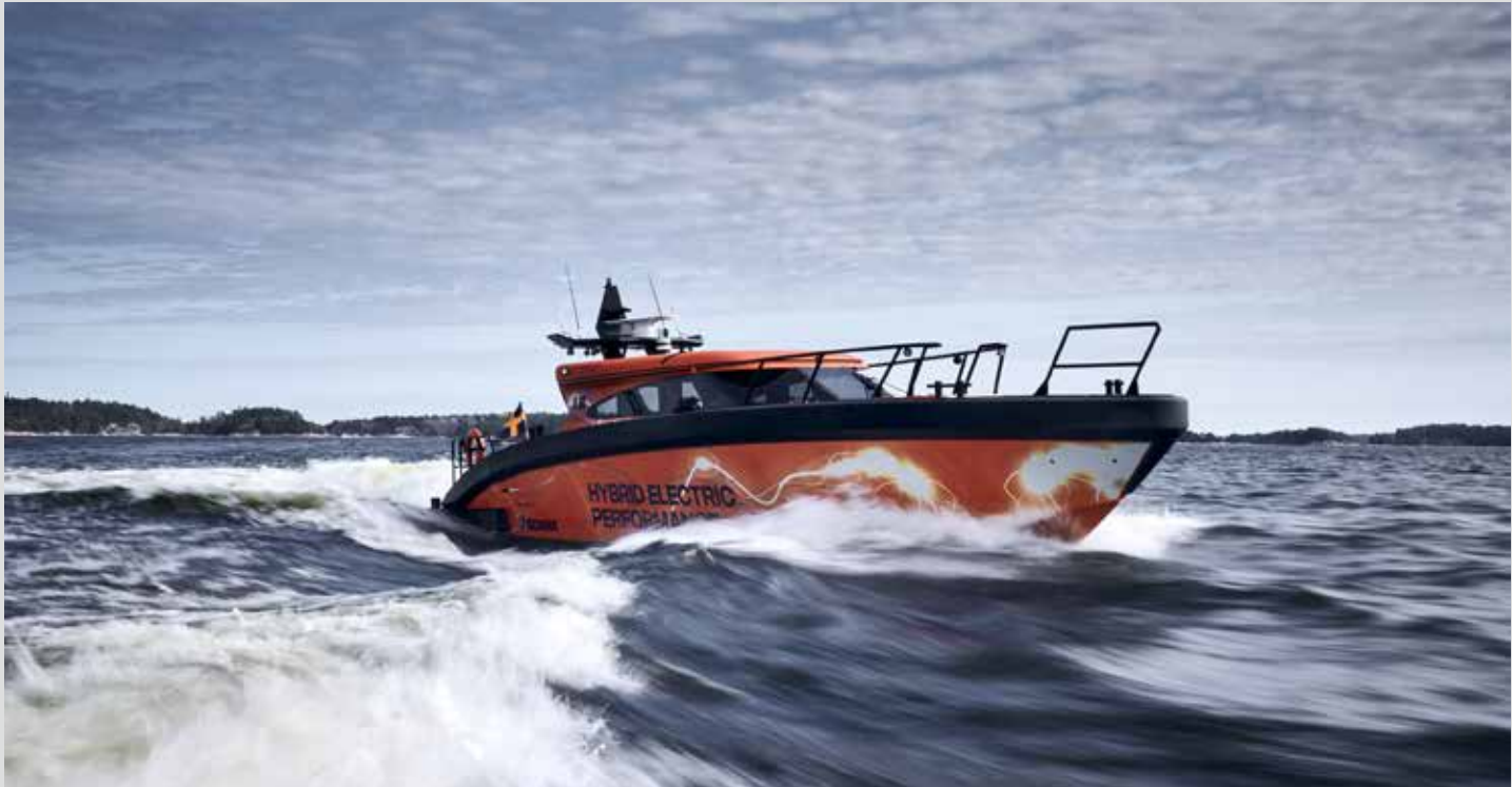
Marell M17 Hybrid Patrol boat with Scania's electrified power systems (e-machine) and two 16 liter V8 engines
