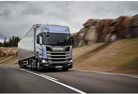
Thanks to a further developed braking system, a front axle that has been located further forward, and a lowered centre of gravity, a typical tractor rig from Scania with a GTW of about 40 tonnes can stop from cruising speed (80 km/h) in a 5 percent shorter distance under normal conditions.
