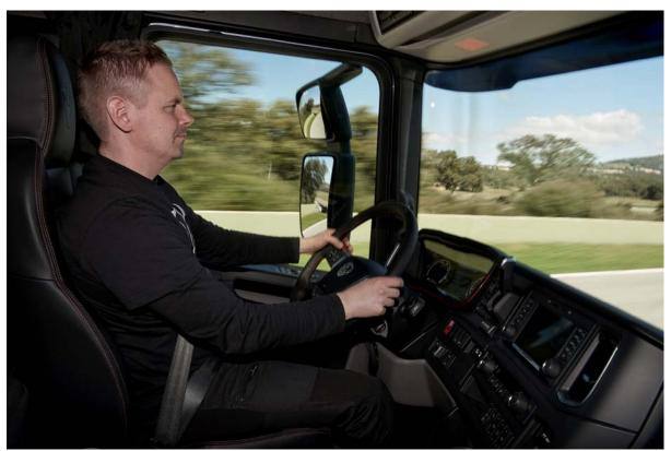
In Scania's new cabs, the driver's seating position has been moved both ahead and out to the side compared with the current range. In addition to greater adjustment scope for the seat, for instance, this also gives the driver an even more commanding overview of the truck's immediate surroundings.
