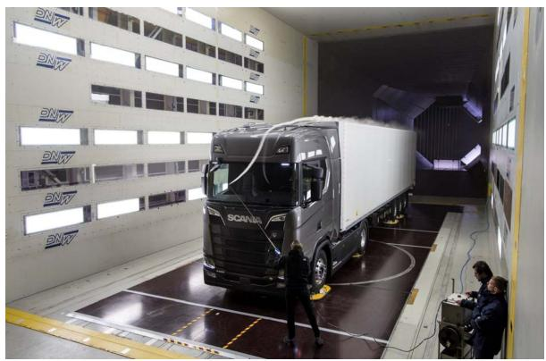
Industry-leading aerodynamics was one of Scania's goals during the development process. Scania has built further on its excellent experiences from the Scania Streamline, and the result is a truck that is so slippery that a long-haul truck can now reduce its fuel consumption by two per cent thanks to lower air resistance.
