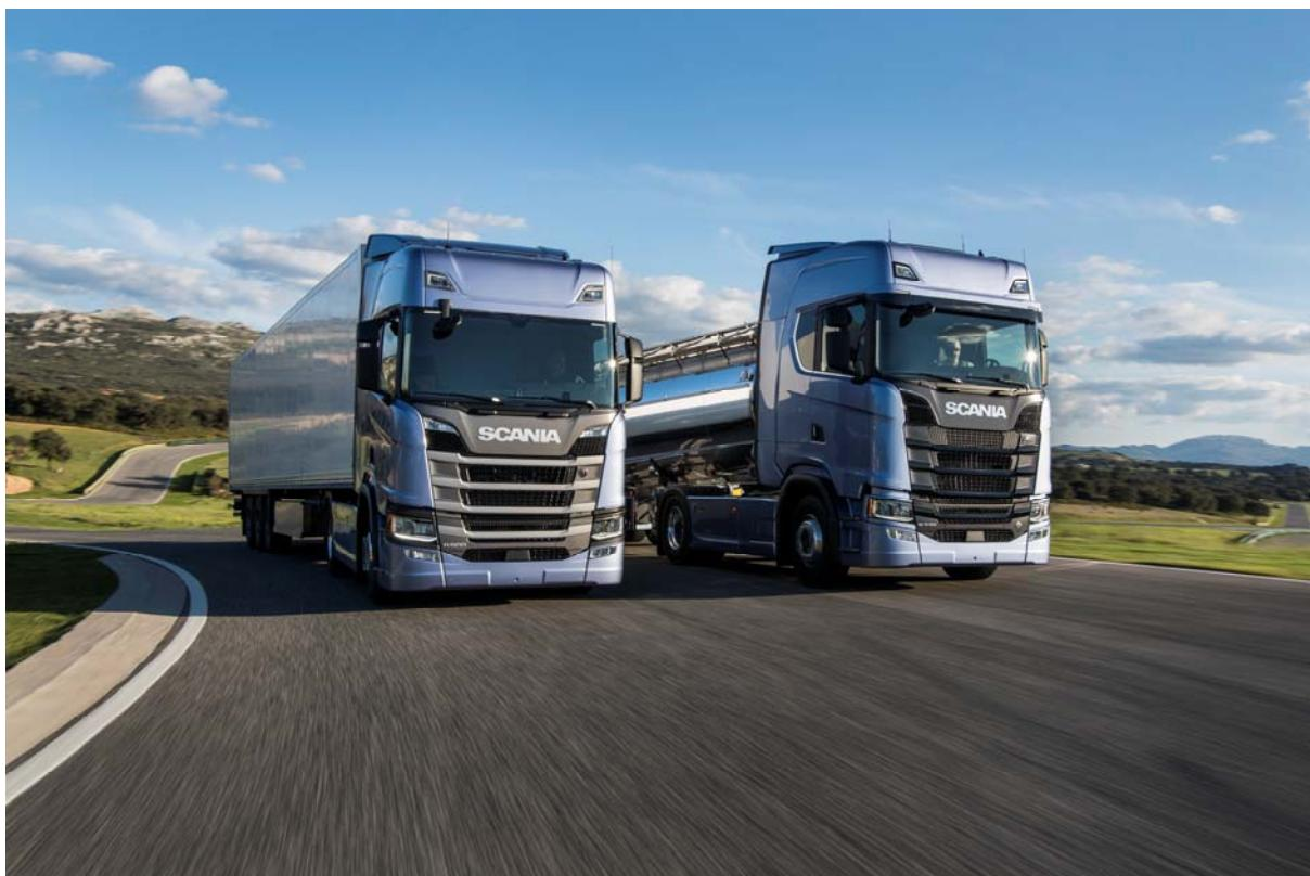
*Scania has the widest range of engines for alternative and renewable fuels in the truck industry. All Scania trucks in the Euro 5 and 6 range, irrespective of generation, can without problem run on up to 100 per cent HVO. In the best-case scenario this can give a CO<sub>2</sub> reduction of 90 per cent compared with diesel.*
