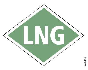
LNG stands for Liquefied Natural Gas. The fuel is cooled to -130 degrees and consists then of liquid and gaseous methane. Leaking LNG boils and expands to 600 times the liquid volume at normal pressure. A vehicle with a full tank can hold up to 180 kg of fuel.
