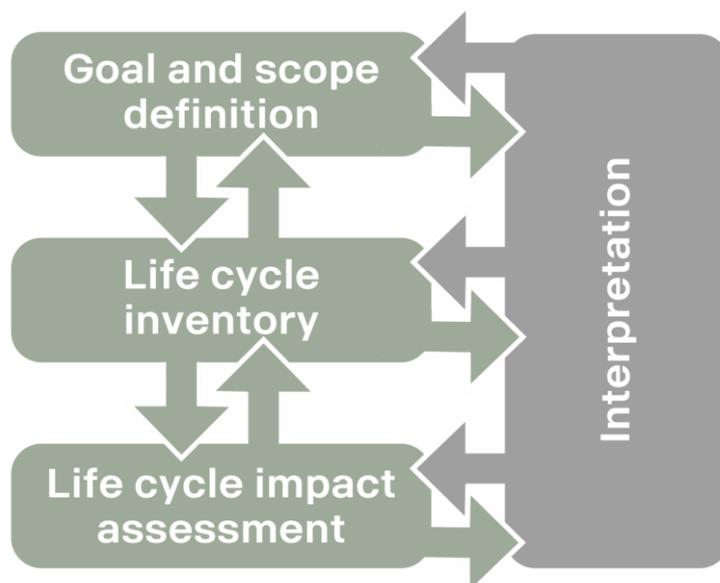
Figure 1. Four stages of the LCA
