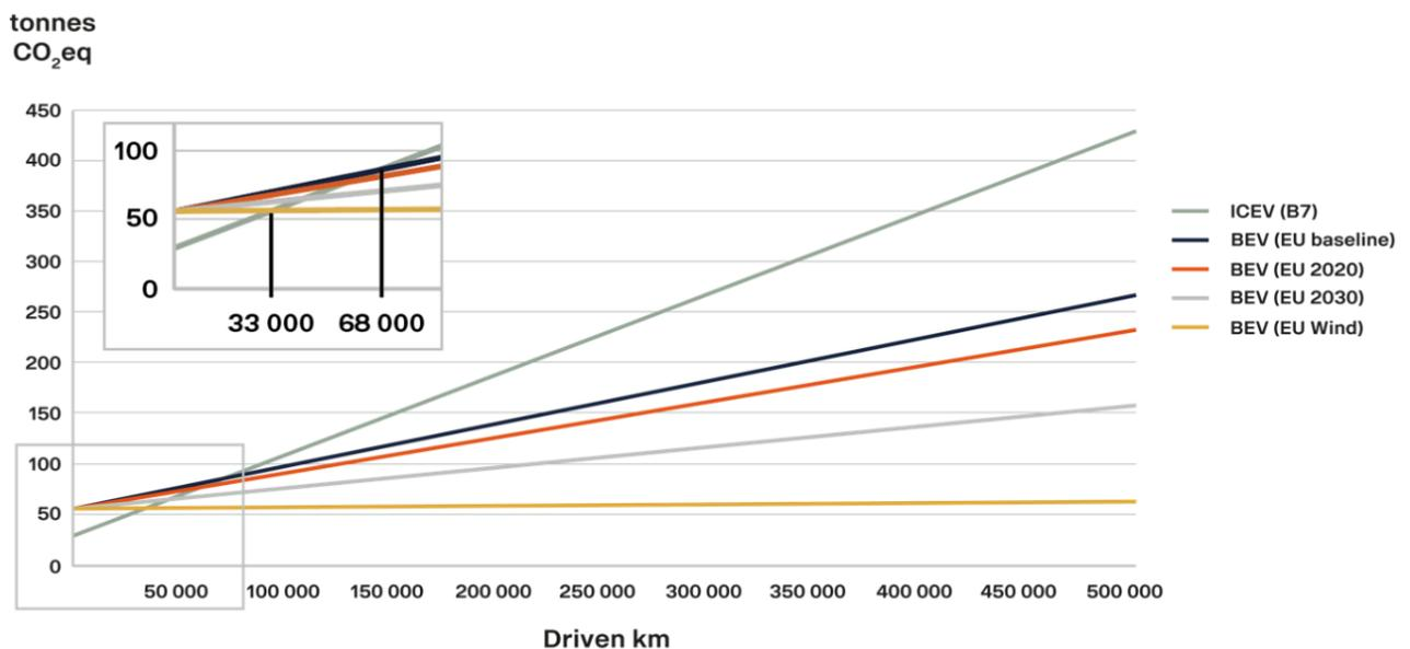
Figure 8. GHG break-even as a function of driven kilometres. The carbon intensity in the grid mix influences when the break-even occurs.
