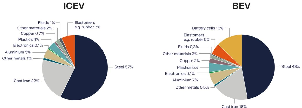
Figure 2. Material composition. Material categories expressed in percent of total vehicle weight.
