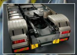
Rear-mounted batteries and the new sideskirts allow more space for fuel tanks holding up to 1,500 litres, even in a short tractor unit.
