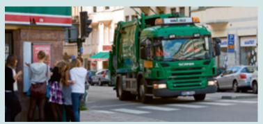
With a low cab that is placed far forward, the P-series allows extra easy entry, for example during refuse collection and local distribution work.
