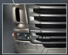
The grille has substantially larger openings between distinct horizontal bars. This underscores a Scania's identity while admitting more air to the radiator and into the engine compartment.
