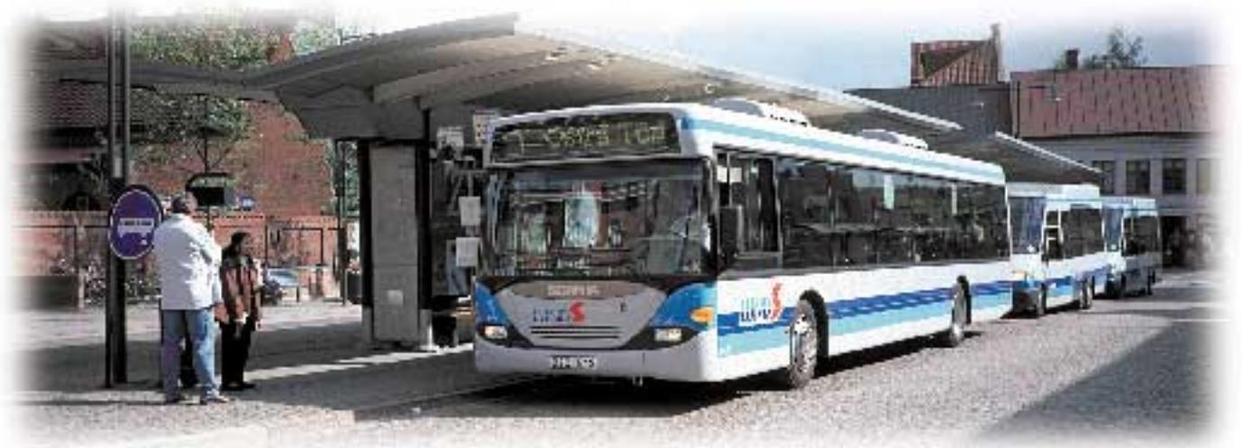
*The OmniCity is Scania's new city bus. It is available either with a body by Scania or as a chassis (N94) on which independent bodywork companies build a customised superstructure.*
