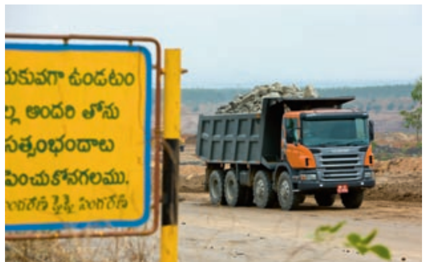
A Scania P 380 four-axle tipper truck being used in an open-cast mine outside of Kothagudem in the Godavari Valley, India.
