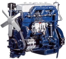
Scania-Vabis' pre-combustion chamber diesel engine featured a compact, 6-cylinder, 7.74-litre design with an output of 120 hp.
